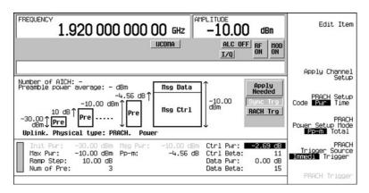
Configure a fully transport layer coded PRACH signal for BER testing
