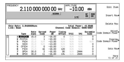
Use the flexible table editor to fully configure a W-CDMA signal waveform
