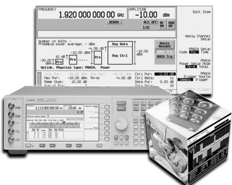
The 3GPP W-CDMA firmware option for the Agilent E4438C ESG Vector Signal Generator provides a broad collection of W-CDMA test signals. Combining the 3GPP W-CDMA waveform playback and real-time personalities into a single firmware option provides a viable test solution for evolving 3G mobile radio networks – from the component to the system level. This simplifies the ordering process and provides a flexible test solution for both development and manufacturing engineers.
