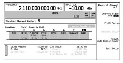
Adjust AWGN as  $E_c/N_o$ ,  $E_b/N_o$  or C/N in real-time
